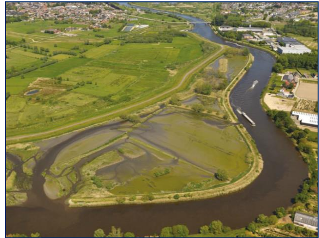
River Scheldt, Belgium; the project area 'Wijmers' being part of the 'Sigmoplan', a river-management plan for flood prevention in combination with nature restoration and navigation. An ecosystem services analysis was used to compare different management alternatives, and the outcome of the societal cost-benefit analysis was used to develop the management plan in the initial concept phase. (© De Vlaamse Waterweg nv)
