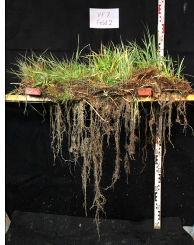
Figure 3.11: Exposed roots of a planting mat with grasses and herbs, installed as bank protection on the River Rhine.
